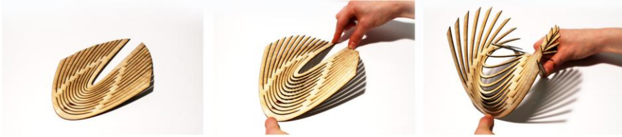
Figure 6. Sequence of operations showing the bending process of plywood at the base of the design concept.
