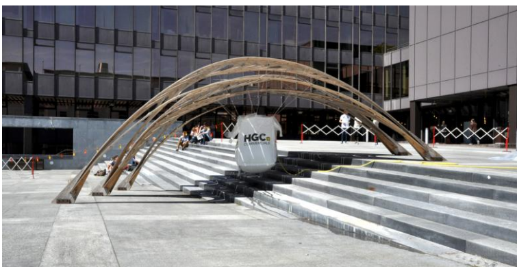
Figure 9. Final load test to validate the efficiency of the lightweight structural system.
