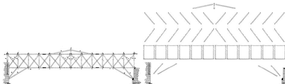
Figure 7. Culmann's description of Long's Truss Frames
