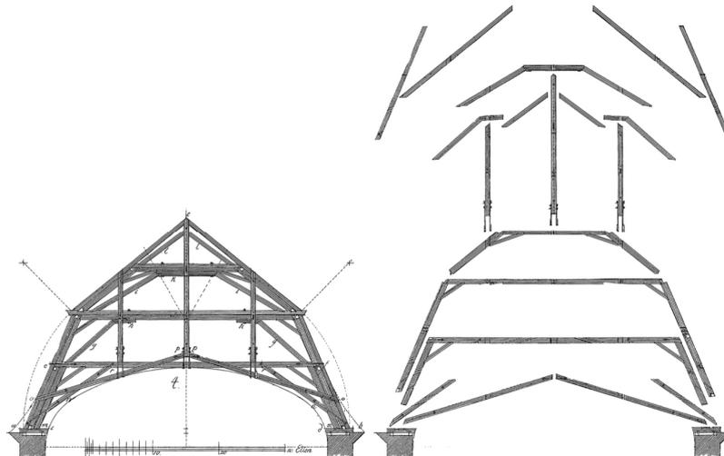
Figure 3. Structural components in Reuss’ gambrel roof
