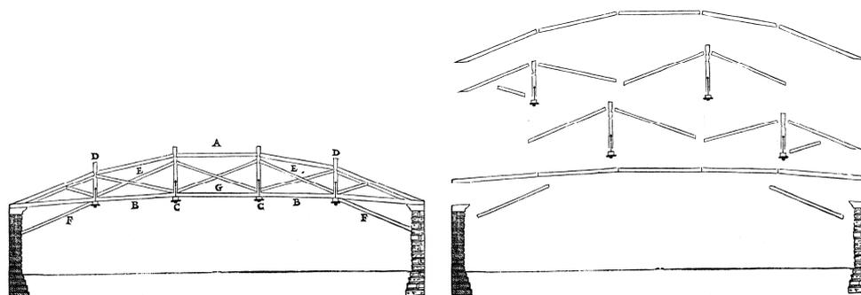
Figure 2. Palladio’s structural description of his 2<sup>nd</sup> bridge concept
