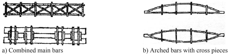
Figure 6. Navier: Composed beams considered as massive continuous beams
