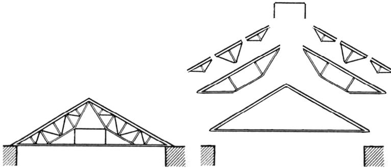
Figure 8. Schwedlers description of a typical conceptual composition for a roof truss
