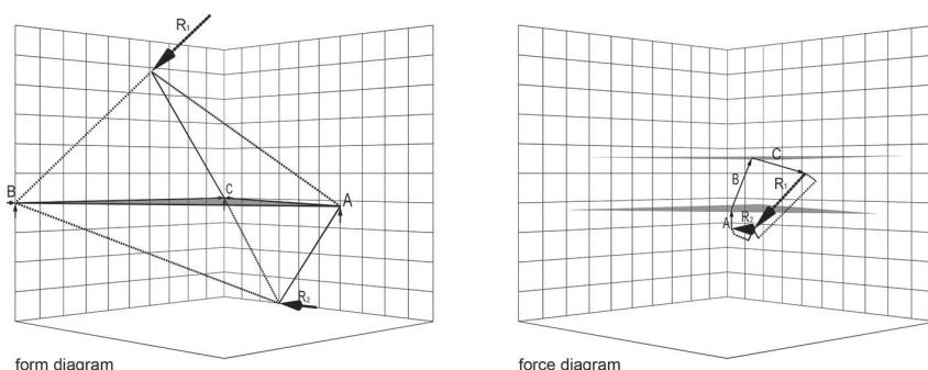
Figure 6. Tetrahedron construction for calculating the support forces.
