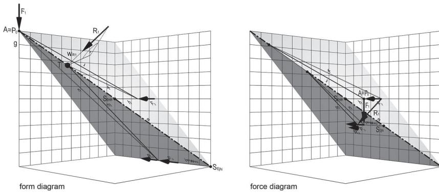
Figure 2. Three skew forces subdivided into  $R_1$  and  $R_2$ .
